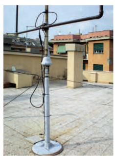
PHOTO 2: Prototype loop pedestal mount, rotator and feed.
