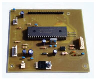
PHOTO 13: Completed PCB for the LED version.
