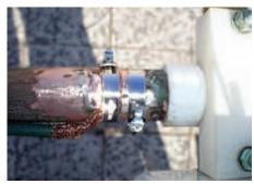
PHOTO 8: Using hose clamps to secure cables to the loop ends.
