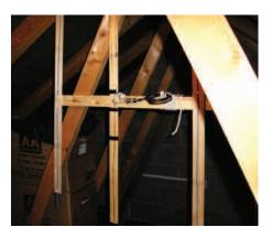
PHOTO 1: The G8PJC 145MHz three-element Yagi located in the loft. The elements are not hard drawn copper so need to be supported on wood battens.
