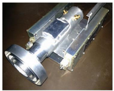
PHOTO 1: Squeezed waveguide horn feed mounted on a carriage designed to fit the existing feed cage on my 2.3m diameter dish. The two side 'blocks' are 6cm solid state power amplifiers.
