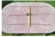
PHOTO 2: The latest edition of my 145MHz three-element Yagi with the elements made from 10SWG (3.2mm) enamelled wire.
