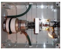
PHOTO 4: Inside the tuning unit. Note the Plexiglass sheet that acts as a chassis and the white Teflon block (see text).
