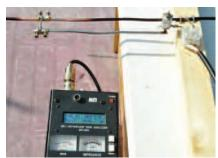
PHOTO 3: Setup for adjusting the antenna gamma match using the MFJ-269.
