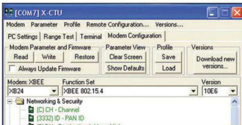
Figure 3. The X-CTU software configures, tests, and communicates with XBee modules attached through a USB port.
