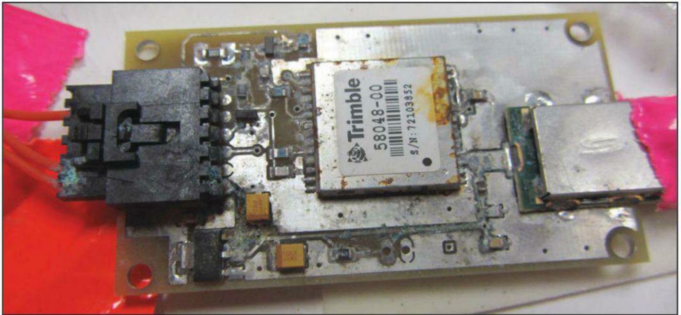
Photo 6. River water and electronics do not mix.
