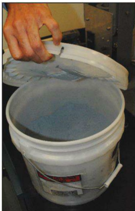
Zinc powder, filtered to a fine mix, ready to be painted on the battery plates in the argon chamber.
