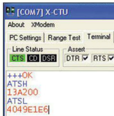
Figure 4. The typed +++ puts an XBee module in AT command mode. The ATSH and ATSL commands fetch the module's serial number.
