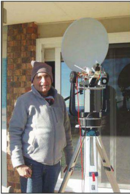
Photo 1. Rex, VK7MO, all set for low absorption losses (low temperature) with 24-GHz system.
