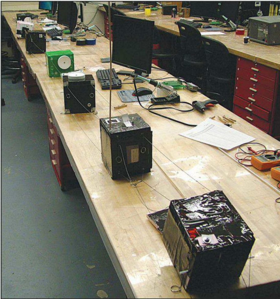
A day or two prior to launch each BalloonSat was tethered to one another and then to the GPS tracking modules. The BalloonSats were tethered together using four thin strings that pass through the plastic tubes that students glued to the inside edges of their BalloonSat.
