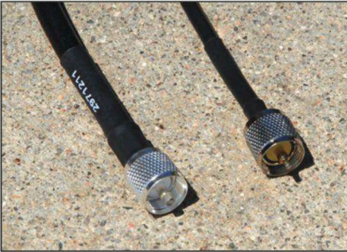
Photo 2. The coaxial cable on the left is the larger and lower loss RG-8 type cable. The cable on the right is RG-8X. Both cables are shown with PL-259 connectors installed.
