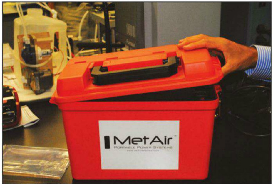
This orange box contains the zinc-air battery ready for deployment simply by pulling the protective shield, letting in air!
