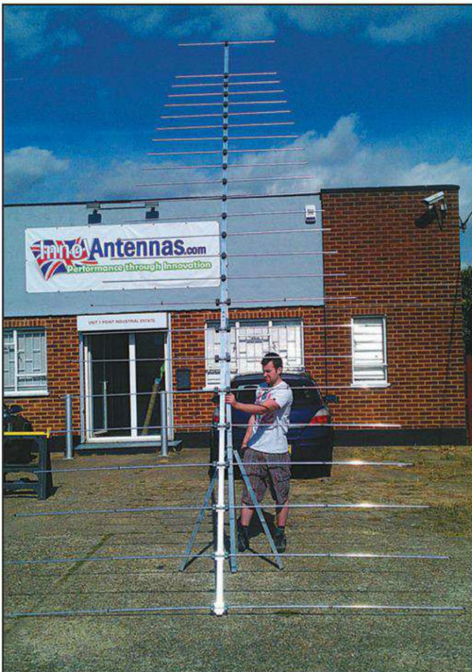
Yes, this is one of InnovAntenna's log-periodic antennas. This particular one covers 48 MHz to 120 MHz and offers a low SWR of 1.3:1 across the entire range.
