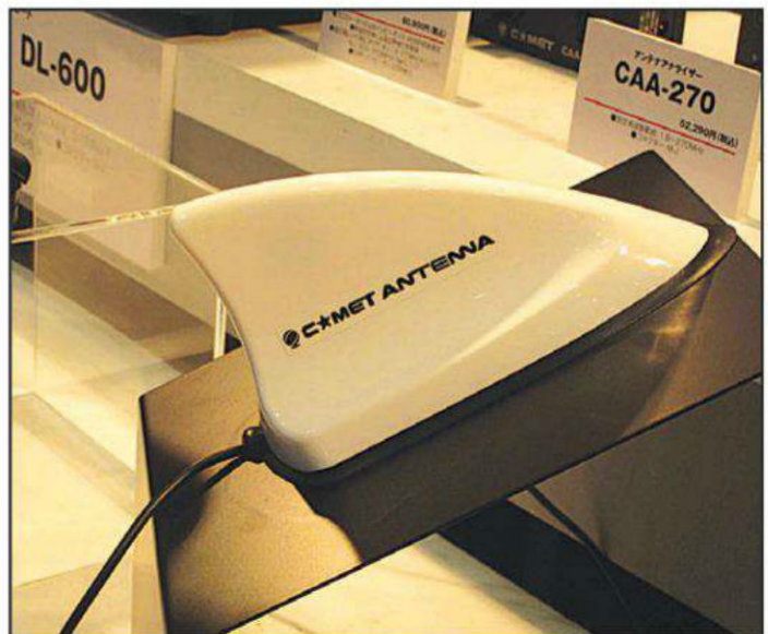
Car makers have made the fin antenna a popular addition to auto rooftops, so why not create a dual-band ham antenna that has the same appearance. This one has a magnetic mount and it's known as the Comet Fin Antenna from NCG, previewed at the recent Japanese Ham Fair and not yet available in the U.S.
