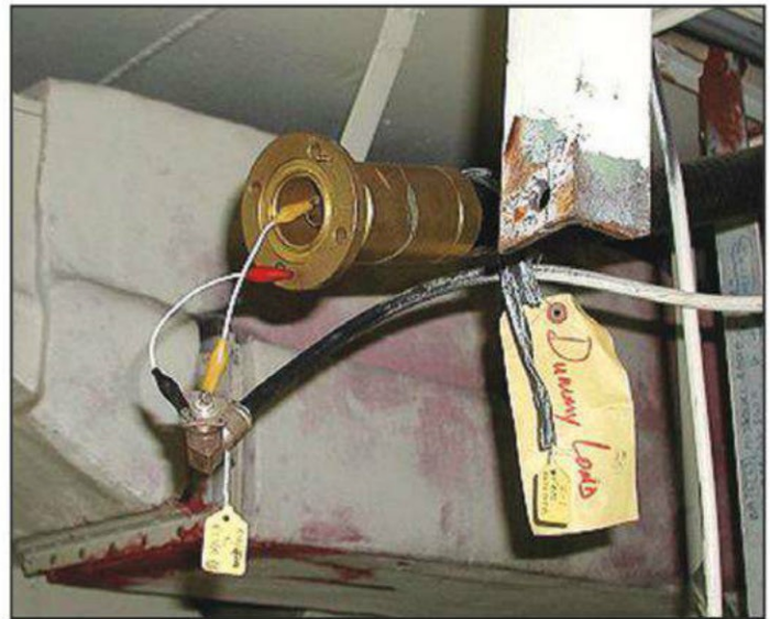
Photo G— In true ham fashion, the output of the TS-450S transceiver is hooked to the ship's 1.5/8-inch hardline with alligator clips!
