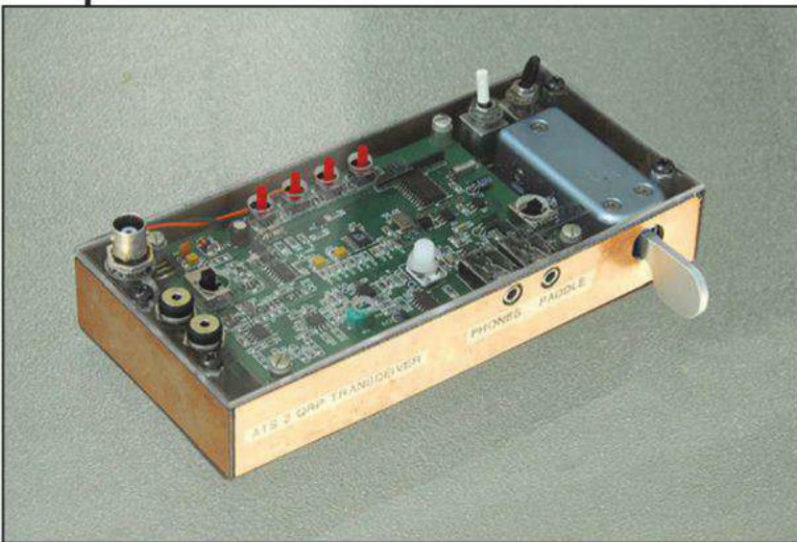
Photo A— This ATS-2 was built and packaged by Steve Russell, N7SR. Steve’s homebrew enclosure includes the transceiver board, a keyer paddle, and battery.
