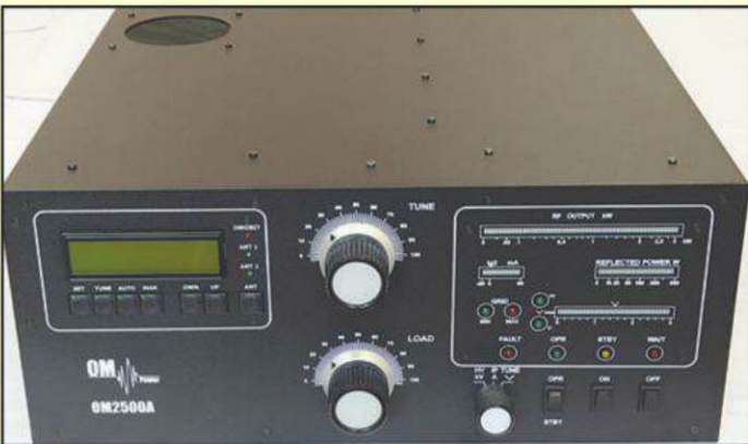
Photo B— The OM-2500A is an automatically tuned kilowatt HF amplifier from OM Power, distributed in the U.S. by Array Solutions.
