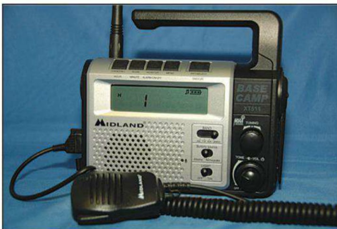
Photo B.— Your “Go-Kit” radios shouldn’t be limited to ham gear. Something such as the C. Crane XT-511 emergency radio (built by Midland) provides reception on the AM and FM broadcast bands and NOAA weather radio, as well as transceiver capability on FRS and GMRS. (K7SZ photo)
