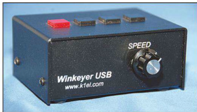
Photo D—The WinKeyer 2 from k1el.com is a great accessory for computerized CW operation. (K7SZ photo)
