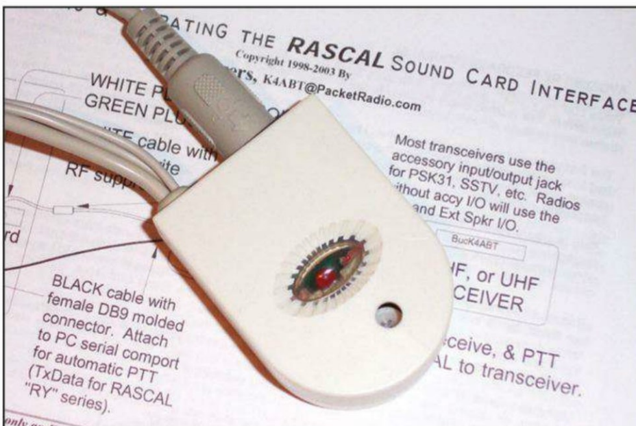
Fig. 4— A basic sound card/radio interface from K4ABT. While the website < www.packetradio.com > can be a little confusing because of the multitude of options, there is very likely a plug 'n play option for whatever radio you happen to have. This RASCAL interface has served me well for several years.
