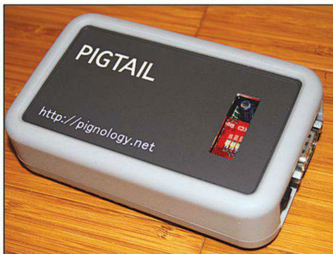
Photo A— Through the use of HamLog 4.0, Pigtail from Pignology LLC gives iOS users wireless control over ham radio transceivers by Icom, Kenwood, Yaesu, Elecraft and others.
