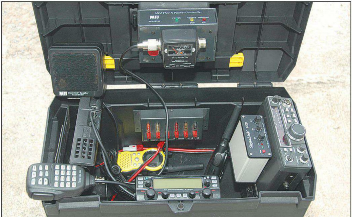
This is Pat's and my Stanley mobile work center box with the current equipment layout that we use for ARES/RACES deployments.
