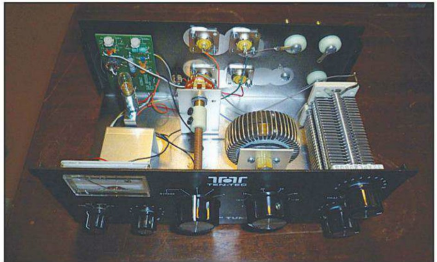
The completed Ten "T" Tuner ready for testing.
