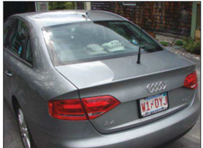
An unobtrusive antenna finishes off this classy installation with a ham plate that adds a nice finishing touch. (W1DYJ photo)
