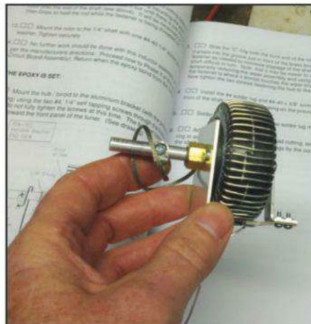
The finished rotary inductor assembly ready for installation.
