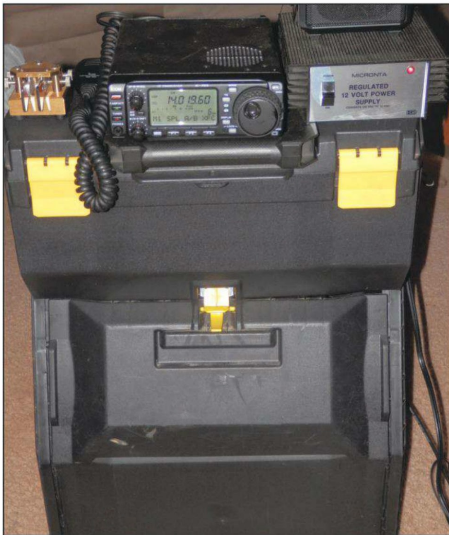
The IC-703 sits atop the Stanley mobile work center. AC power supply is located to the right of the radio and the mic/CW paddles are on the left. See text for details.
