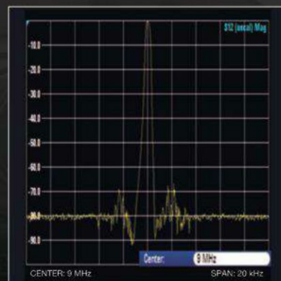
Characteristics of the Crystal Roofing Filter (300 Hz)
