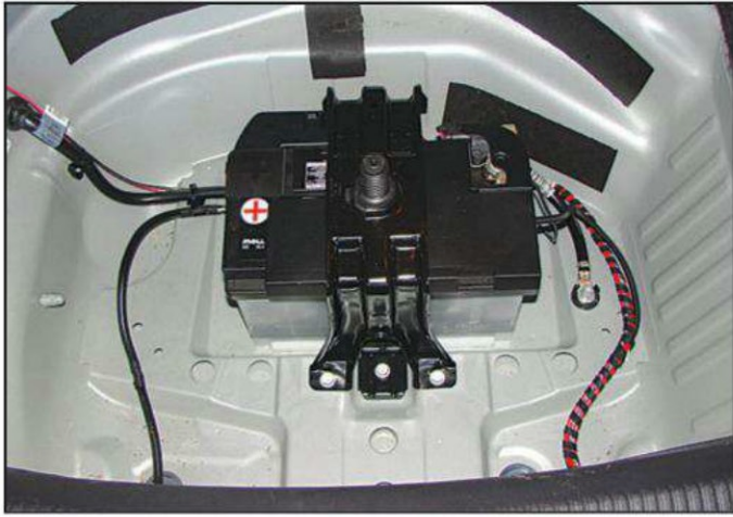
The battery is buried below the spare tire in W1DYJ's Audi. Routing power to the transceiver doesn't get much easier! (W1DYJ photo)
