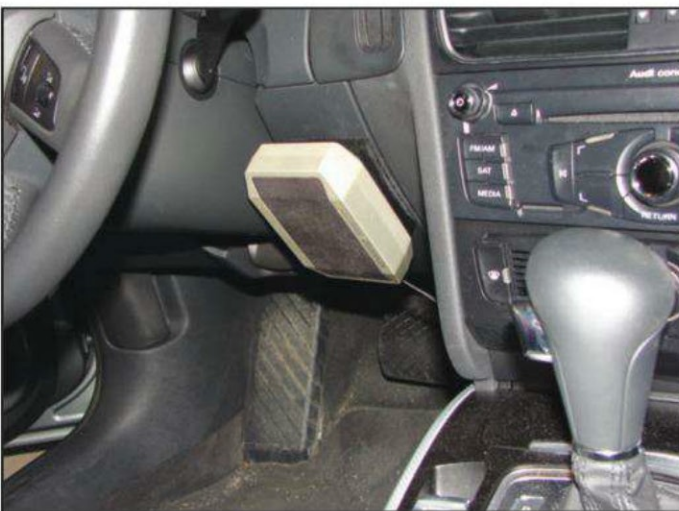
This speaker location is easily heard, yet away from other vehicle controls and some distance removed from the airbag deployment zone. (W1DYJ photo)
