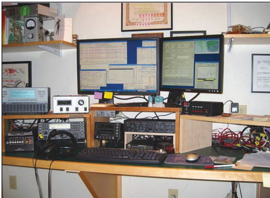
This is the operating table at W2LK. Les operates SO2R using two Elecraft K3 radios. The empty space on the right is for the second K3 but the radio is at Elecraft at the moment. Also, the SPE 1K amp on the left will be on the right and an Alpha 9500 will be in that spot when the K3 gets back. (Photo Courtesy of Les Kalmus W2LK)
