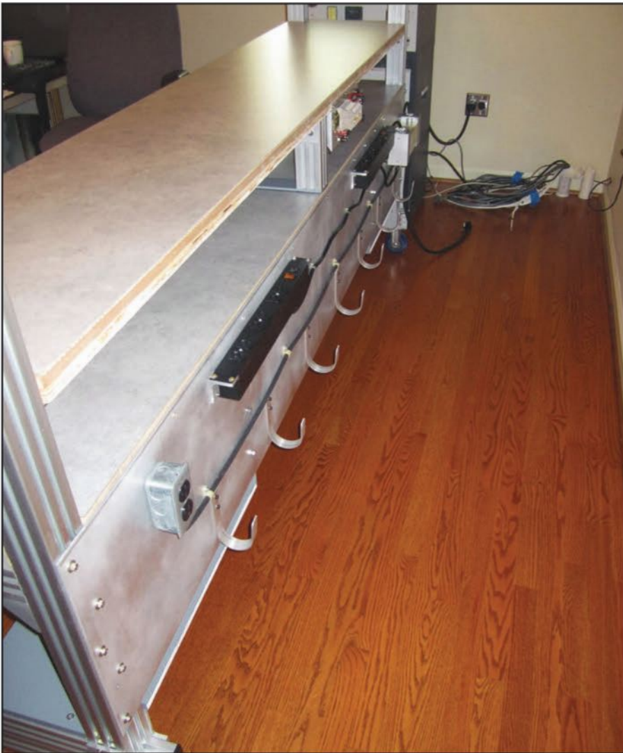
The back wall has dedicated power outlets and a mains filter, all controlled by one master switch on the front leg. In addition, Dubovsky fabricated some wide aluminum hooks to aid in cable management.
