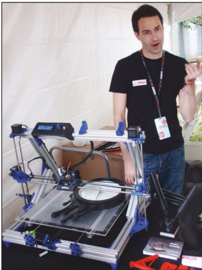
gMax president and founder Gordon LaPlante speaking about the gMax printer prototype < http://www.gmaxprinter.com/ > he showed at Maker Faire 2013. As a Kickstarter campaign, supporters pledge a certain amount of money to be on the list to receive one from the first batch of kits. The large (16" x 16" x 9") print volume is one of the attractions of this model, as is the extensive use of off-the-shelf parts and its ability to make prints directly from an SD memory card, without a computer. A pledge of just under $1200 gets you a complete kit when they start shipping in early 2014.
