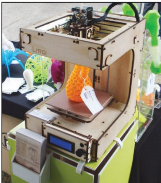
The Litto, from Tinkerine Studio in Vancouver < http://www.tinkerines.com/ >, is a smaller printer made from laser-cut plywood. You can get it as a kit for just under $1000, or fully assembled for $300 more. Weighing only about 13 pounds, it redefines "portable." Print resolution is a reasonable 100 microns, and the print volume is a moderate 5.3" x 4.7" x 7.9". Tinkerine also offers its larger Ditto+, essentially the same printer but with a larger print volume.
