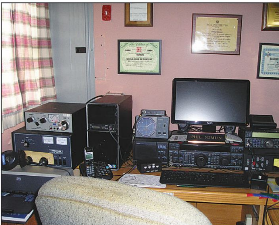
Here's a simple shack setup at N2MUN. Note the equipment stacking and close-in location of the important controls such as his rotator controller. (Photo courtesy Phil Lewis, N2MUN)
