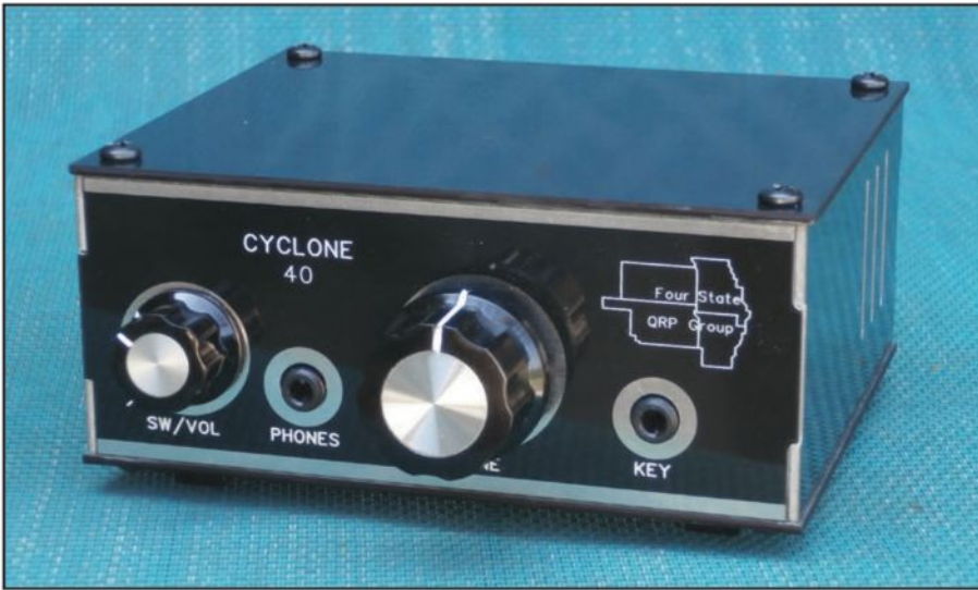
Photo G. The Cyclone 40 kit from the 4 State QRP Group. All of the cabinet pieces snapped apart from one sheet of PC board material.
