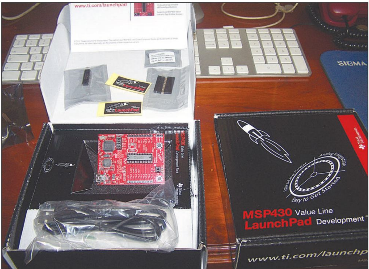
Photo A. The basic Texas Instruments LaunchPad kit comes with a PC board, two microcontroller chips, a USB cable, one 32-kHz crystal, and some stickers.
