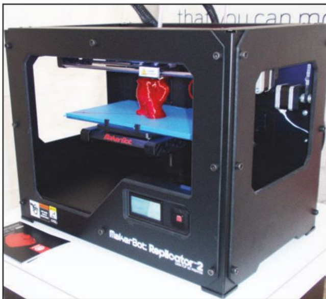
The Replicator2 from MakerBot < http://www.makerbot.com/ >, one of the biggest names in 3D printing. Fully-assembled, the Rep2 runs about $2200, features a build volume of about 11" x 6" x 6", but lacks a heated bed, so it can only print PLA (polylactic acid) plastic. The Replicator2X ($2800) is available, but "only for true daredevils and experimenters," per MakerBot. The bundled software runs under Windows®, Linux, and Mac, and the support team is top notch.
