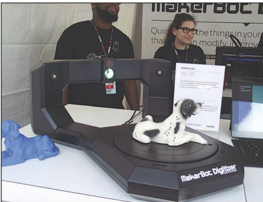
Photo I. The MakerBot "Digitizer" 3D scanner lets you make a computer model of virtually any solid object. The file can then be fed to a 3D printer for replication.
