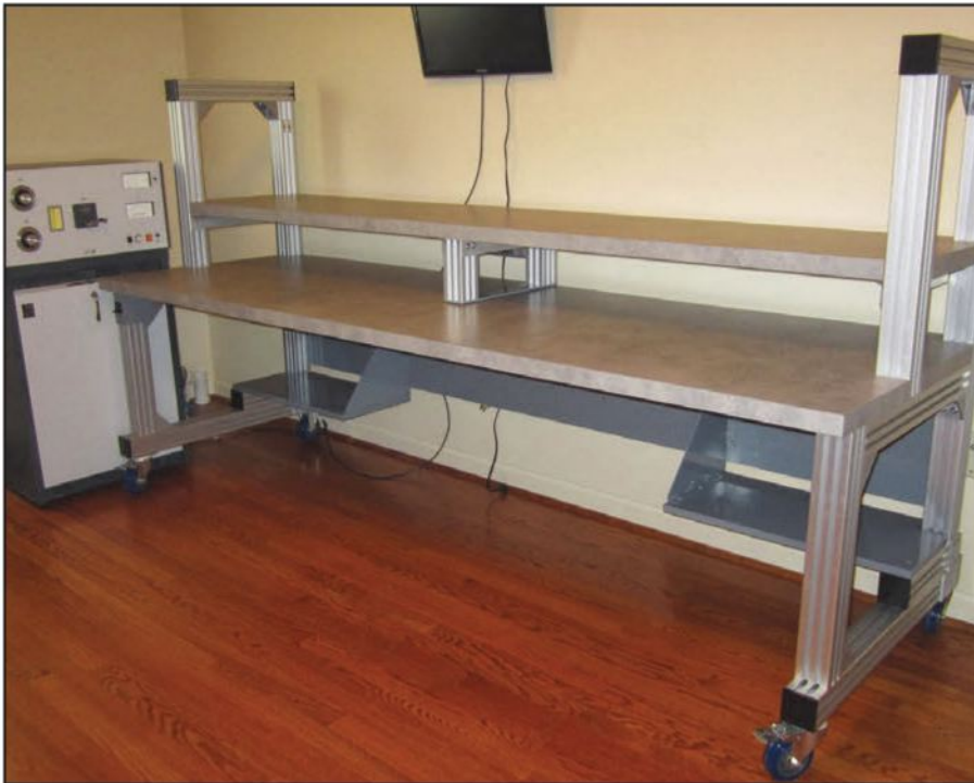
N4UA's table features more horizontal equipment location and less vertical "stacking." The table is 8 feet wide and 30 inches deep, with one full-width 18-inch shelf above the radios. Notice the total-locking casters. These casters lock not only the wheel on the axle; they also lock the vertical axis of rotation. The table can be rolled away from the wall for access to the cables and backs of the equipment. Also, note the two small shelves underneath for power supplies and such.
