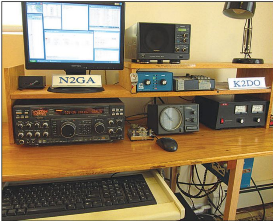
Here's the author's temporary operating table. The tabletop is handmade from red oak that was routed and then coated with polyurethane so the front edge is rounded not to chafe the arms. Note the keyboard drawer to allow typing at the correct height and the computer monitor located at an ergonomically correct eye level. Antenna selection is via an Array Solutions Six Pack with the controller mounted close to the operating position and the cable connection box mounted under the table. The antenna rotator is also within easy arm's reach. (Photo courtesy of N2GA)
