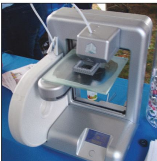
The Cube by Cubify 3D Systems < http://cubify.com >. This is a truly plug-n-play product, targeted toward users who just want to design and print, rather than tweak and experiment. Printing in both ABS (acrylonitrile butadiene styrene) and PLA, its 5.5-inch cubical print volume is large enough for most things you'll ever want to print. This printer has built-in WiFi, so you don't even need to use a cable. The base machine starts at around $1300. Cubify also sells the CubeX, which features higher resolution, up to three print heads and a larger print volume.
